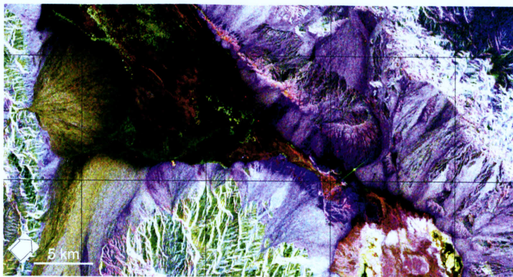
Fig. 2. Dozens of fans are visible in this Shuttle Imaging RADAR (SIR-C) composite image of northern Death Valley. The colours refer to the signal wavelength (L-band 24 cm; C-band 6 cm) and polarization, or orientation of the electric field (HH, horizontal emission and horizontal detection; HV, horizontal emission and vertical detection): RGB = LHH, LHV, CHV (24, 24, 6 cm). The large fans to the west are yellow, indicating a strong signal return in the red and green channels. This is a result of large cobbles and blocks near 24 cm in size. Blue fans in the east and south have many particles close to 6 cm in size, interspersed with fines, which are smooth to the synthetic aperture radar signal and appear dark. The valley floor is dark because of smooth sediments (the Mesquite dune field is the dark deposit in the centre) and evaporites, green from scattering and polarization changes by vegetation and red from scattering by subsurface, longer wavelength features such as layering. SIR-C image courtesy of NASA/Jet Propulsion Laboratory.
