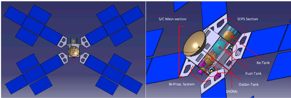
Fig. 10. E<sup>2</sup>T baseline proposed configuration of the spacecraft. Left panel shows an enlarged view of the S/C and right panel shows a close-up view of the spacecraft.
