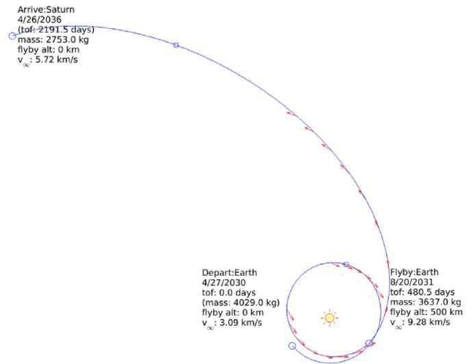
**Fig. 8.** Interplanetary transfer to Saturn. Red arrows indicate electric propulsion thrust. (For interpretation of the references to colour in this figure legend, the reader is referred to the web version of this article).
