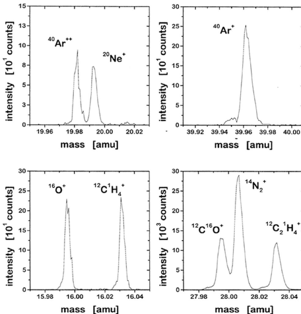
Fig. 5. Separation of isobaric interference such as occur at 16, 20, 28, and 40 u/e for the indicated species is possible based on heritage of RTOF/ROSINA from the Rosetta mission (Scherer et al., 2006; Wurz et al., 2015).
