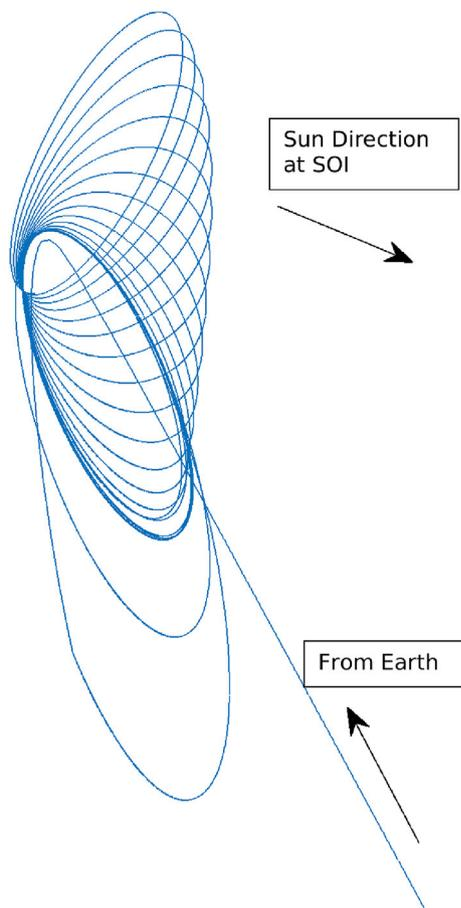
Fig. 9. Sample tour with two period- and inclination-management Titan flybys followed by a science phase with 6 Enceladus flybys and 17 Titan flybys (Inertial representation).
